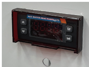
Figure 6: Push controller into the hole. Silicone will seal against mounting surface.
